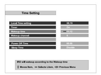
Use the ((,,)) buttons when selecting the On/Off mode. If the Timer menu Timer menu is set to On, the Wakeup Time Menu, the Wakeup channel Menu and the Power Off Time Menu becomes adjustable.
